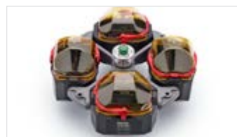
TX-1000 rotor for up to 196x 5/7 mL blood tubes
